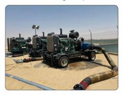
Dewatering Centrifugal Pumps (100-3000 M3/hr.)
